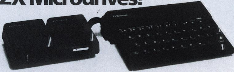
They're here at last - the spectacular ZX Microdrives. And as promised they deliver tremendously fast access to gigantic amounts of program and data on ZX Microdrive Cartridges. Microdrives are controlled by the new ZX Interface 1, which also provides an RS232 peripheral interface and sets up a local area network (the ZX Net) of anything from 2 to 64 Spectrums!
